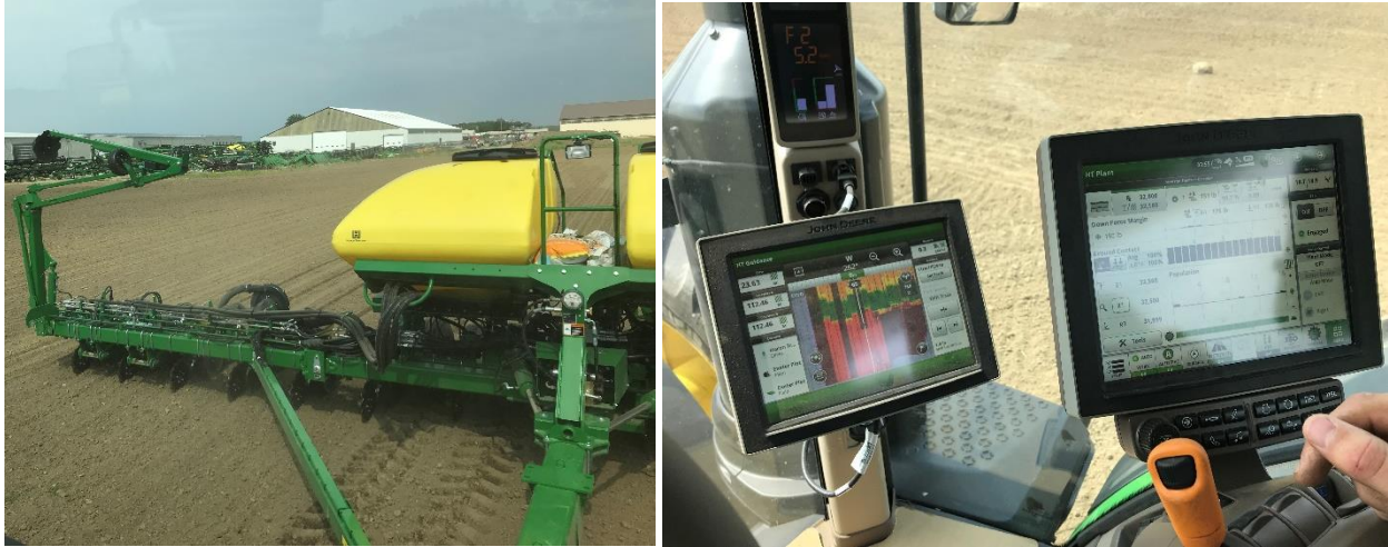
Figure 5: Technology utilized to plant variable rate soybean demonstration plot. Left hand images shows 1775 MaxEmerge 5e, with independent electric motors on each row. Right hand image shows the Prescription operating on the Gen4 4600 Command Center and Extended Monitor integrated in the 8295R tractor
